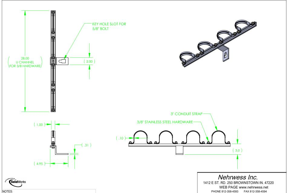
NW-28-3XXXX is a fixed standoff that holds four 3" conduits 3" off pole. The bracket is aluminum with 3/8 stainless steel hardware. It has a single key mounting hole for 5/8 bolt
