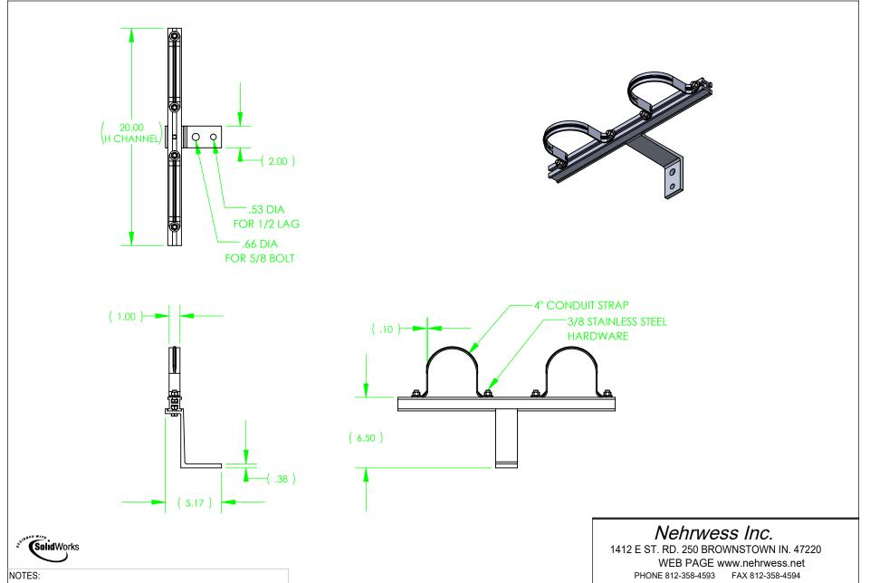
This is a fixed bracket that stands the conduit 6.5" off the pole. The bracket is aluminum with stainless steel hardware. There are two mounting holes one for 5/8 bolt one for 1/2 lag.
