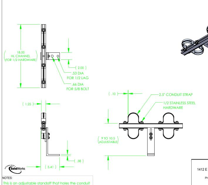
9 to 10.5" off the pole. The bracket is aluminum with stainless steel hardware. There are two mounting holes one for 5/8 bolt one for 1/2 lag.
